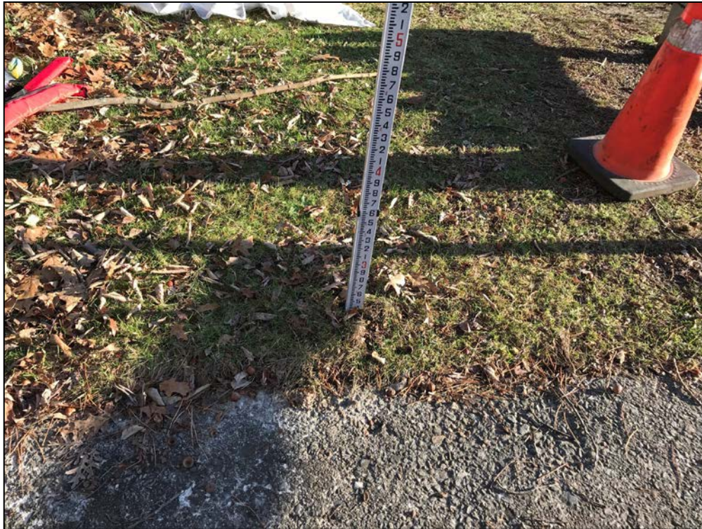
Photo No. 9: Sinkhole behind right training wall probed to 2.4 feet.
