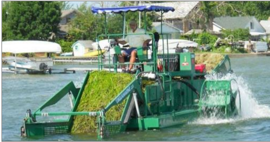
A mechanical harvester collecting cut submerged vegetation for upland disposal.
